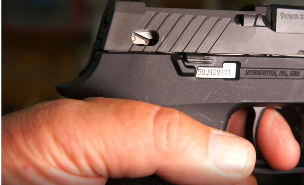
The firing pin block disengaging with less than .075” of a trigger pull under less than 1.5 pounds of pressure. See Appendix F.
