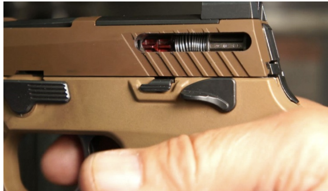
Exposed striker on a P320 (M17 model) with the striker under tension
