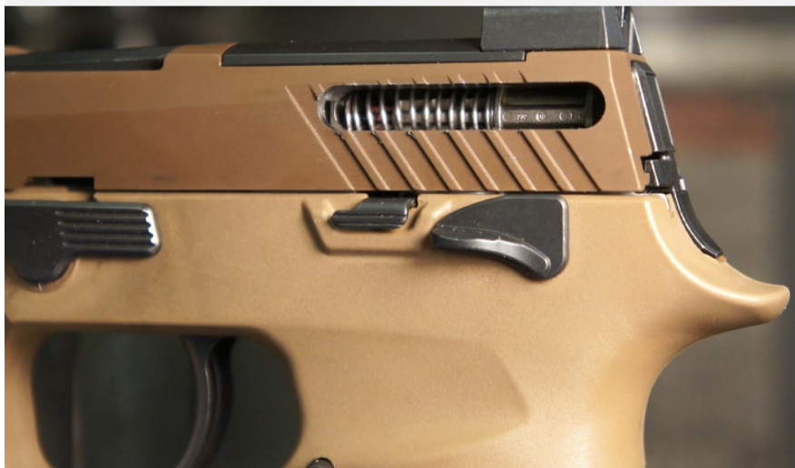
Exposed striker on a P320 (M17 model with manual safety included)
