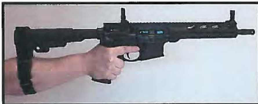
Submitted firearm with SBA3 accessory in the extended position, used in accordance with the manufacturer's stated intent to "stabilize" the firearm.
