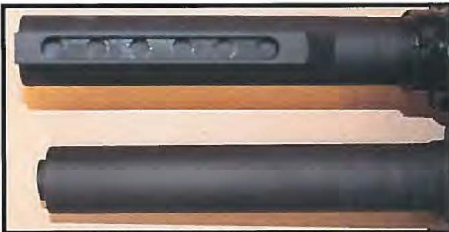
Submitted Sample with Mil-Spec Receiver Extension (top) compared to Sample Round Pistol Receiver Extension (bottom)
