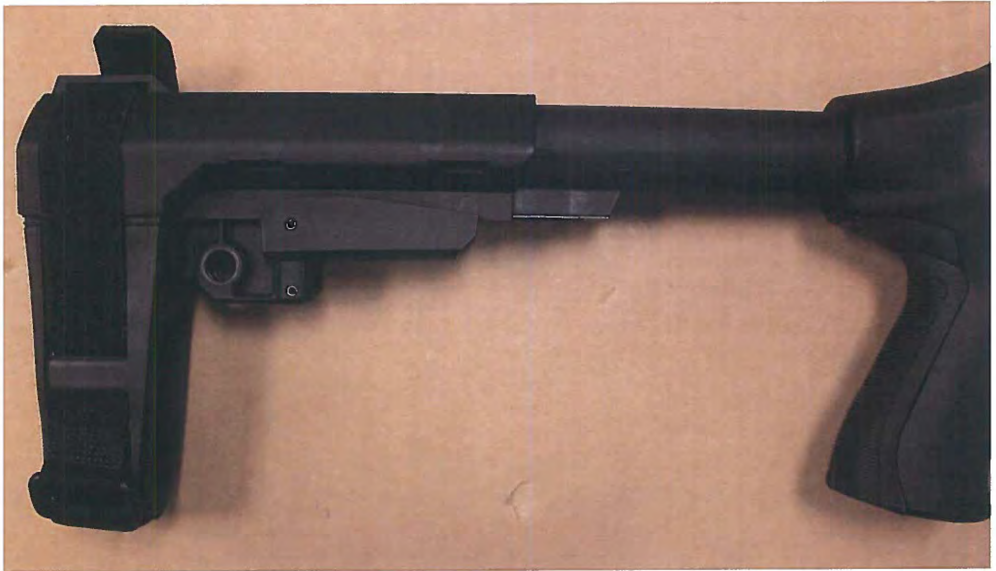
Exhibit 13 SBA3 accessory installed onto Carbine Receiver Extension
